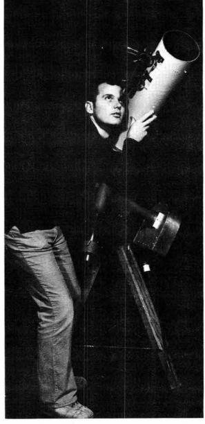
BILL WAMPLER zeroes in on a deep-sky object with his 6-inch Newtonian reflector. He built the telescope when he was in high school—the instrument has an equatorial mount and clock drive.
